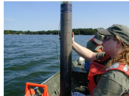
A sediment core is extracted from the bottom of Lake Ripley in 2007.
